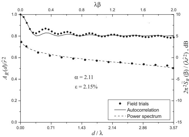
Fig. 4. Empirical versus theoretical normalized autocorrelation and normalized power spectrum functions (indoor measurements).
