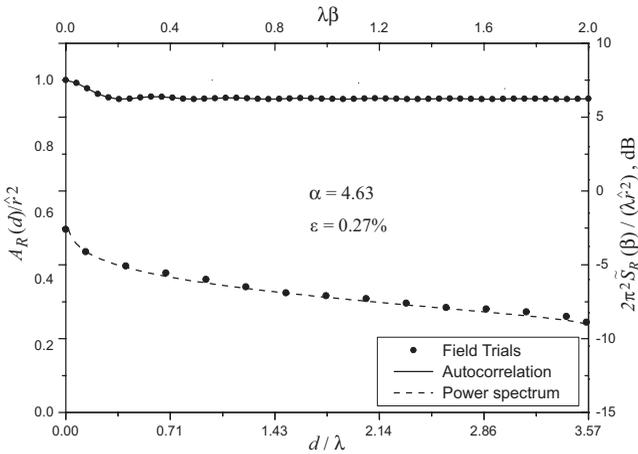
Fig. 5. Empirical versus theoretical normalized autocorrelation and normalized power spectrum functions (outdoor measurements).
